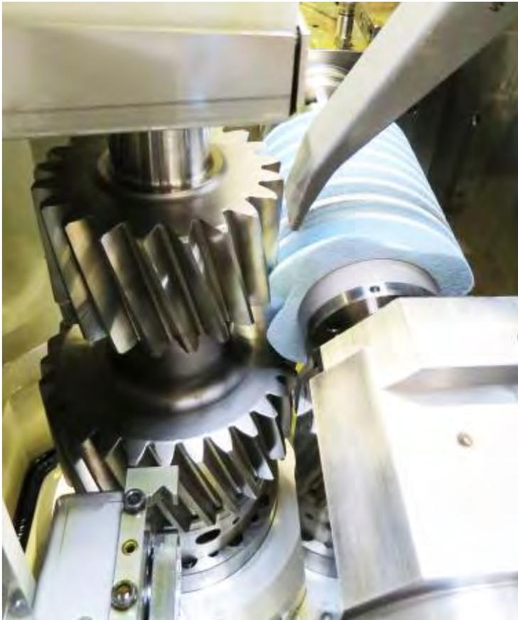
**Image 1:** Generating grinding of a gear with interference contour
