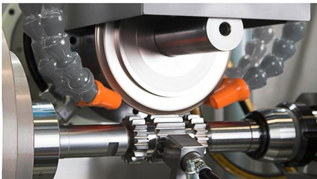
**Figure 5: Machining of a triple pinion © KAPP NILES**
