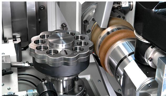
**Figure 1: External cycloid machining on the KAPP NILES Gear Centre KX 300 P © KAPP NILES**
